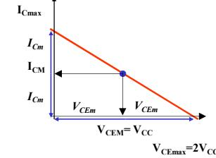
$$\eta_{max} = \frac{P_k}{P_{CC}} = \frac{\frac{1}{2} V_{CEm} I_{CM}}{V_{CC} I_{CM}} = \frac{1}{4} \frac{V_{CC} I_{DM}}{V_{CC} I_{DM}} = 0.25$$
