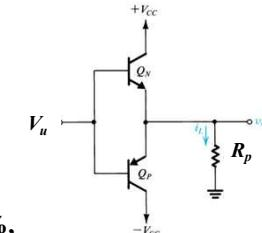
$$[V_{CC} > 22.9V, I_{pmax} = 2.25A, P_{CC} = 32.8W, \eta = 61\%, P_{dn} = P_{dp} = 6.7W]$$
