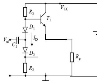
$$J_{Dm\max} = J_{Bm\max} + V_{um\max} / R_2$$
