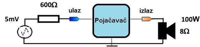
$$P_z = v_z \cdot i_z = v_z \cdot \frac{v_z}{R_z} = \frac{v_z^2}{R_z} = 100W$$
