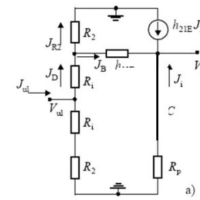
$$\text{Naponsko } A = \frac{V_i}{V_{ul}} \approx 1$$
